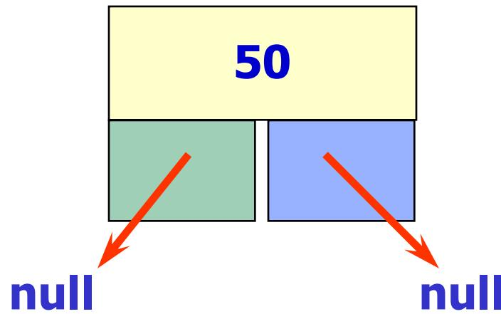
**A tree node typically has a data component and a reference to a left child and a reference to a right child.**
